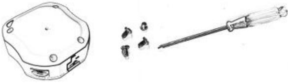
5.1.2 Forward push and open the metal piece, put the SIM card into the card slot, and press the metal piece to its original position, push it backward.
